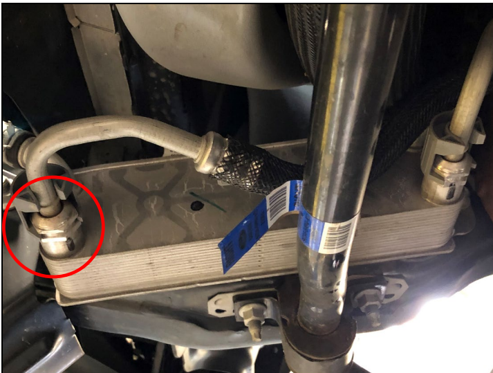
FIGURE 15 – Stock Trans Cooler – Outlet Marked
