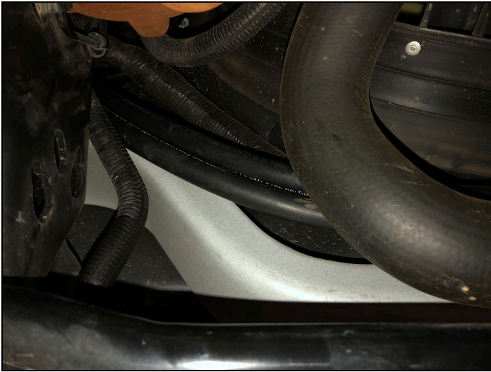
FIGURE 20 – Cooler Hoses Tucked Above Core Support
