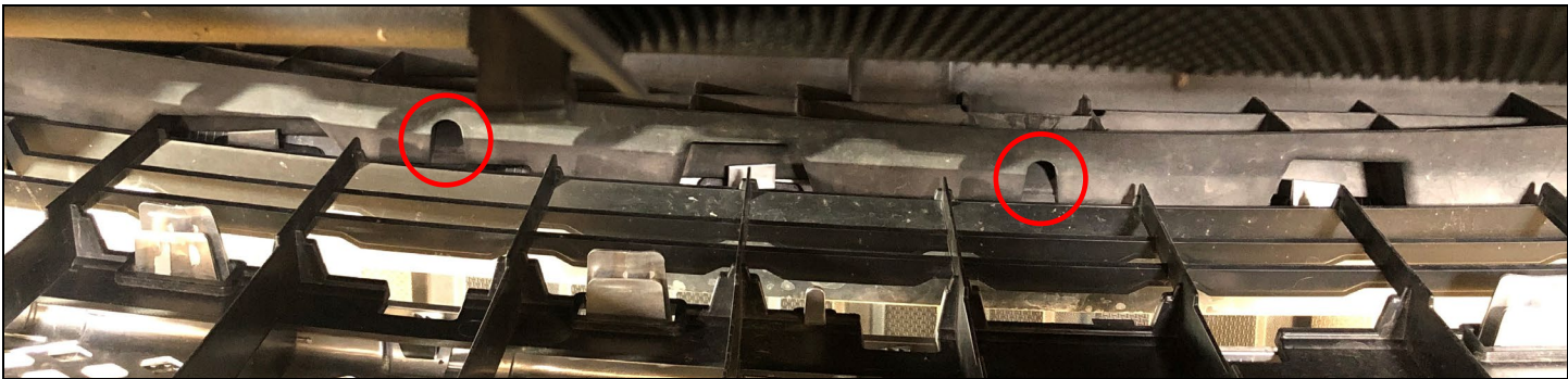
FIGURE 2 – Lower Grille Retention Clips (only 2 of 5 pictured)
