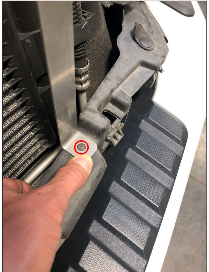
FIGURE 5 – Marking Hole Location
