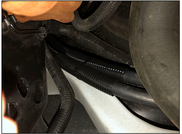
FIGURE 21 – Protective Loom and Cable Tie on Hoses
