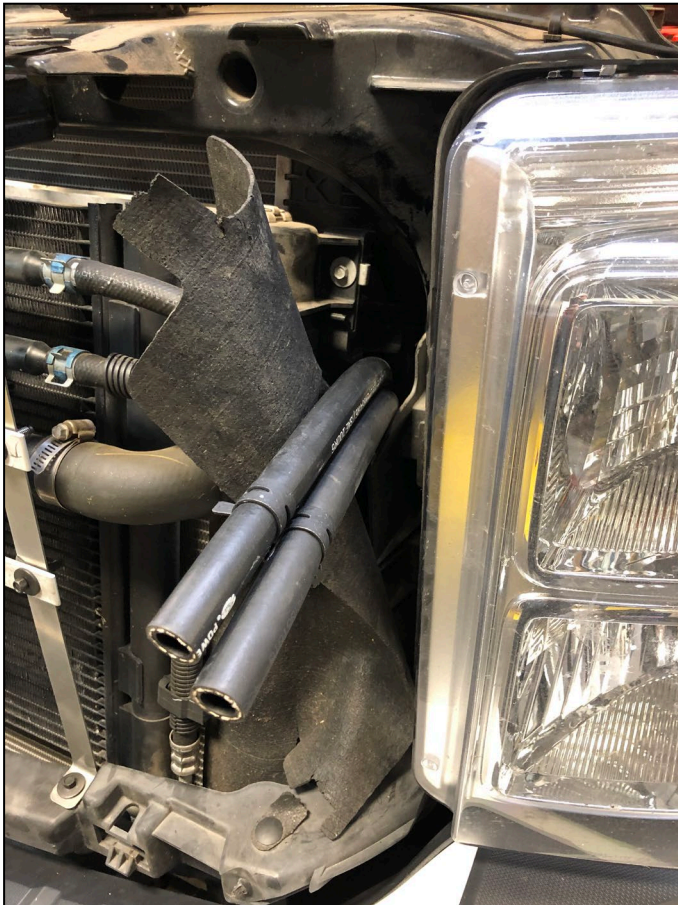
FIGURE 9 – Driver Side Hose Routing Location
