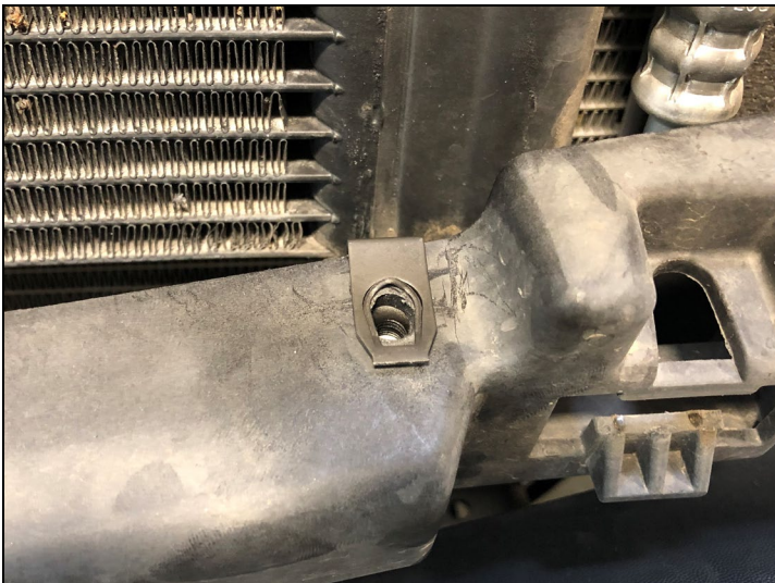
FIGURE 6 – Hole Drilled & Clip Capture Nut Installed
