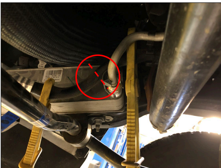
FIGURE 17 – Hose Pinch Pliers Installed On Outlet Hose
